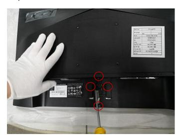
Step.3 Separate hooks between MID\_FRAME and R/C
