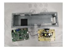
Step.8 Remove connecter cable and separate main board and power board, separate mylar and shielding
