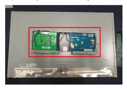
Step2. Insert 30 pin LVDS FFC to LCM, then use acetate cloth tape to tape FFC.
