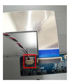
Step6. Insert 30 pin LVDS FFC to main board. Use AL tape to fix. (Tape in blue circle)
