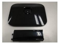
Step.14 Remove six silicon rubbers and unscrew one screw
